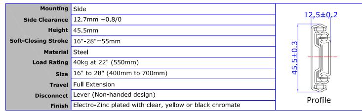
All Dimensions are in Millimeters (mm)
